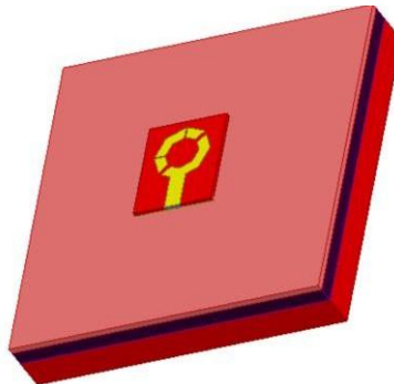
Fig 9. Antenna on a planar human tissue model
