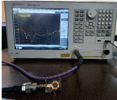
Fig 8. Fabricated antenna and measurement setup
