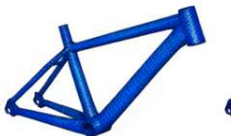
Finite element mesh applied to the bicycle frame for numerical analysis.
