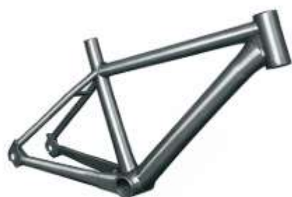
3D CAD model of bicycle frame used for finite element simulation.
