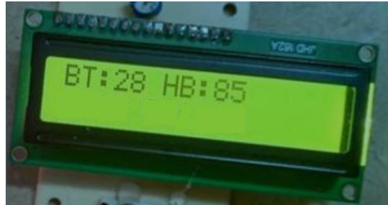
Fig 4. Heart beat sensor values displays on LCD
