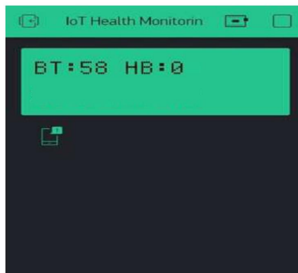
Fig 9. Low body temperature triggers an alert on the Blink app
