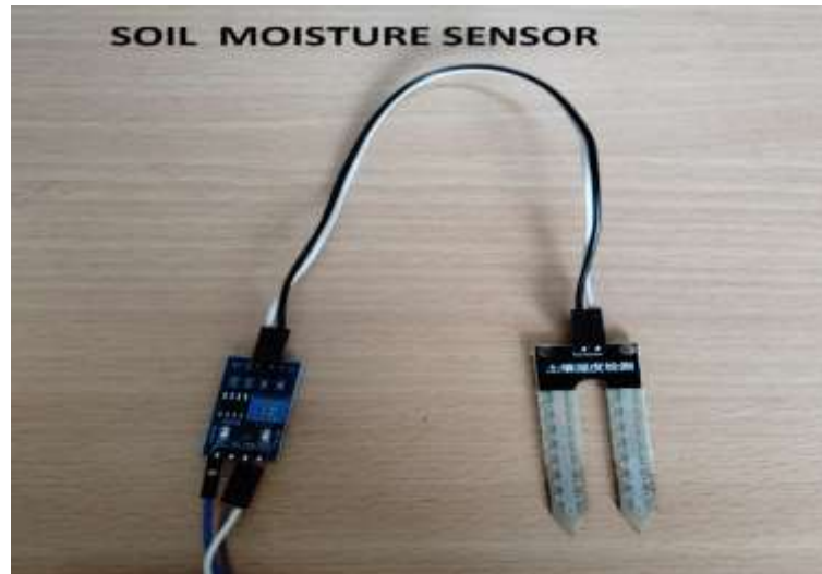
Fig. 4. Soil Moisture sensor interfacing circuit.
