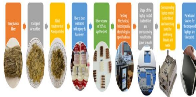
Fig 4.2. Stages involved in the process of contriving laptop panels & sleeves
