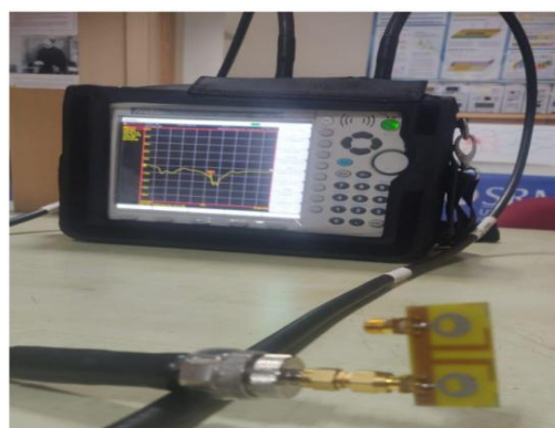
Fig 11. Experimental Setup Utilized for Conducting the Testing of the Proposed Antenna.
