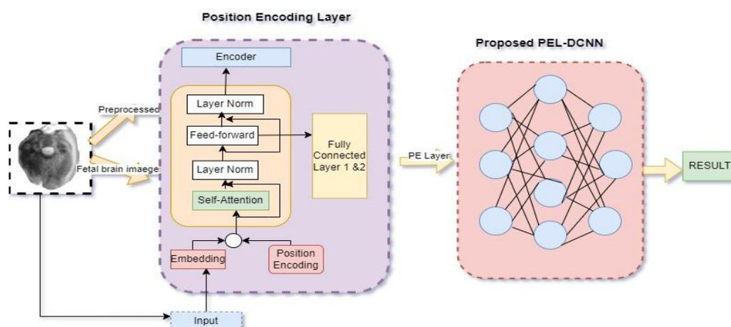
Figure 4. Our Proposed Architecture for combining Position encoded Layer and Deep Convolutional Neural Network
