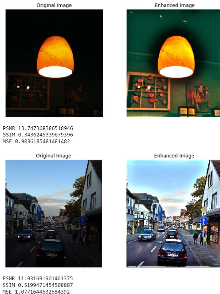
Fig. 3: Illustrating the obtained enhanced Frames using proposed model with quality metrics as PSNR, SSIM, and MSE.
