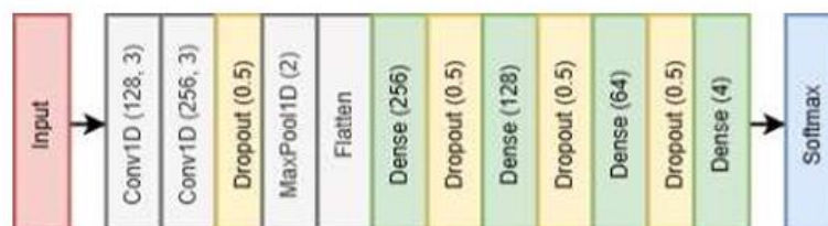
Figure 2: CNN Experiment Model Architecture
