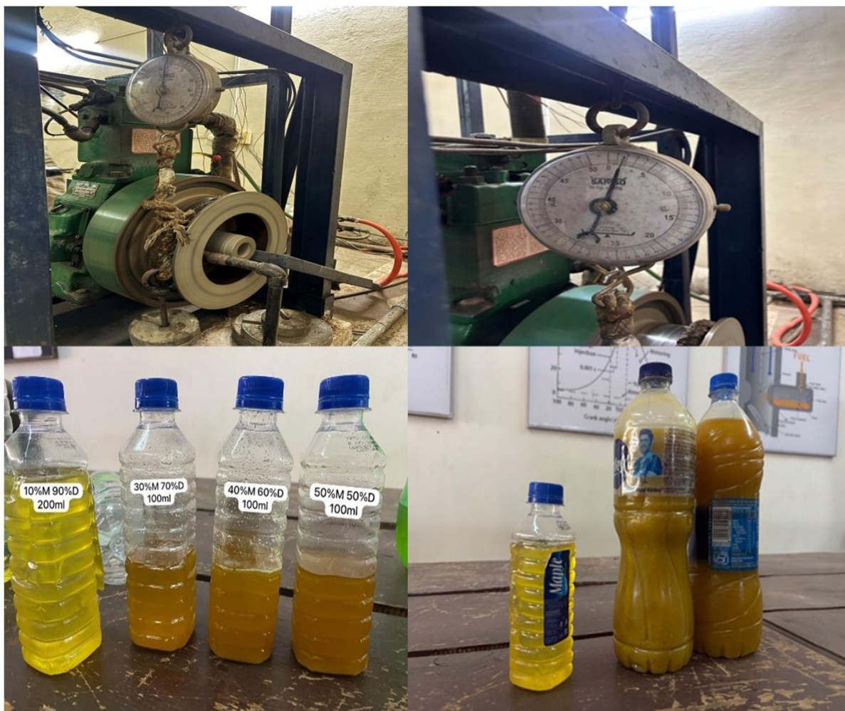
Fig. 1.(a) Diesel Engine Sample of Diesel Blends with Mahua Oil (b) Spring balance dynamometer (c) Sample of Diesel Blends with Mahua Oil (d) Blend and Mahua Oil
