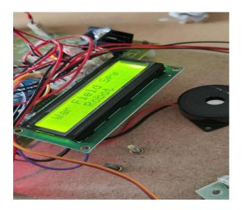
Here the circuit is turned ON by giving the regulated power supply of 12v which is converted to 5v dc current. The LED is the indication for 5v current so, if there is 5v current then automatically the LED glows. The generated 5v dc current passes to every hardware component in the circuit.
