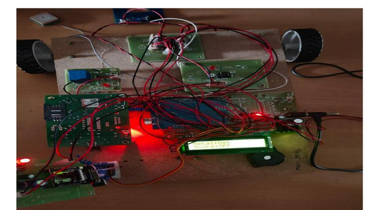
The LED shows the Metal and Smoke detection. When the metal is detect the LED displays "Det" and the metal is doesn't detect it displays the "OFF". When the smoke is detect the LED displays the "Det" and the smoke is doesn't detect the LED displays the "OFF". Same as above figure.
