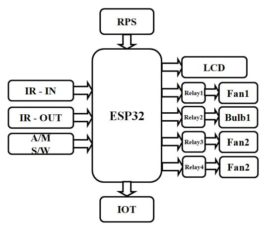
The above block diagram consists of IR-IN, and IR-OUT sensors which sense the persons entering and exiting the auditorium .And provided with two mode switch either automatic or manual mode, ON-OFF switch also given at input side.
