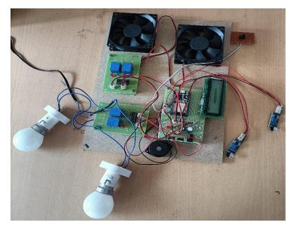
The above image shows the hardware equipment of the project. The kit is turned ON by giving the regulated power supply of 12v which is then converted to 5v dc current. The LED is the indication for 5v current so, if there is 5v current then automatically the LED glows. The generated 5v dc current passes to every hardware component in the circuit
