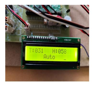
The LED displays the Temperature and humidity levels and mode switches on LED by sensing the grain humidity values. We can see in the above placed picture how the values are represented.
