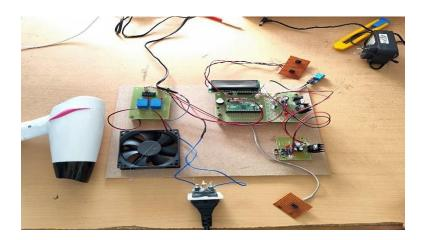
Here the circuit is turned ON by giving the regulated power supply of 12v which is converted to 5v dc current. The LED is the indication for 5v current so, if there is 5v current then automatically the LED glows. The generated 5v dc current passes to every hardware component in the circuit.
