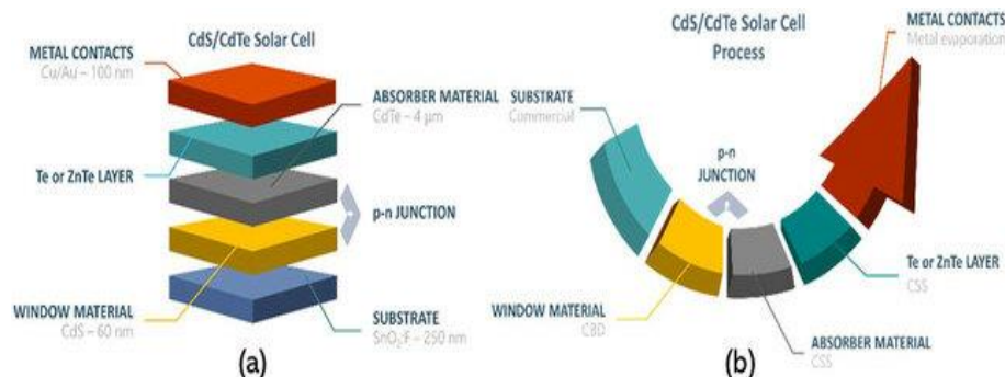
Fig.1(a) CdS/CdTe solar cell structure
