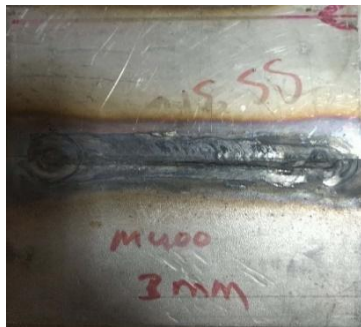
Fig. 3: FSW dissimilar welded joints of Monel 400 and SS 316L and tool wear.
