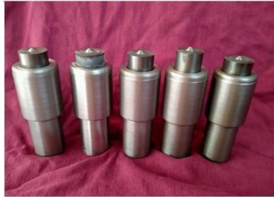
Fig. 1: FSW tool dimensions CAD diagram Fig. 2: FSW tools machines with diamond grinder
