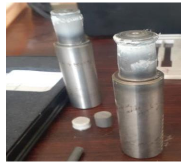
Fig. 3: FSW dissimilar welded joints of Monel 400 and SS 316L and tool wear.
