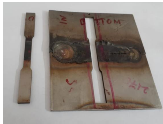
Fig 8: UTM results of S3 and FSW joint of Monel 400 vs SS 316L
