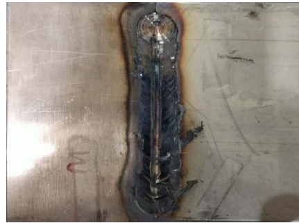
Fig. 3: FSW dissimilar welded joints of Monel 400 and SS 316L and tool wear.
