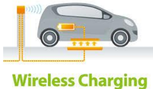
Figure:1 Wireless charger for EV
