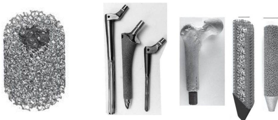
Figure 7: AM-EBM fabricated Ti-6Al-4V complex objects with a Software models[68]
