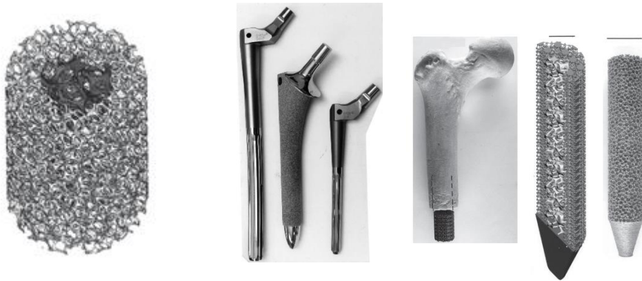
Figure 7: AM-EBM fabricated Ti-6Al-4V complex objects with a Software models[68]
