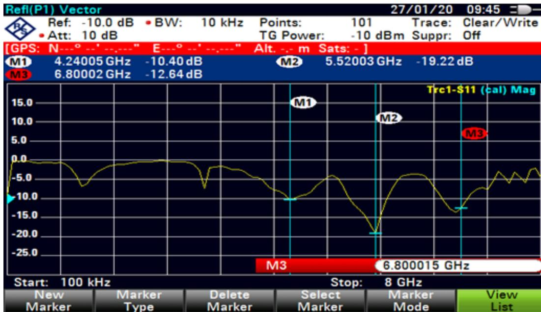
Figure 6. Experimental result using ZVH8 Vector network analyzer
