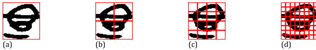
Figure 6: Character Images: (a) one zone (b) four zones (c) sixteen zones (d) sixty four zones
