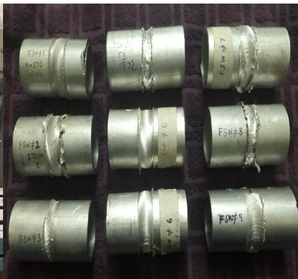
Fig.2 Friction stir welded samples
