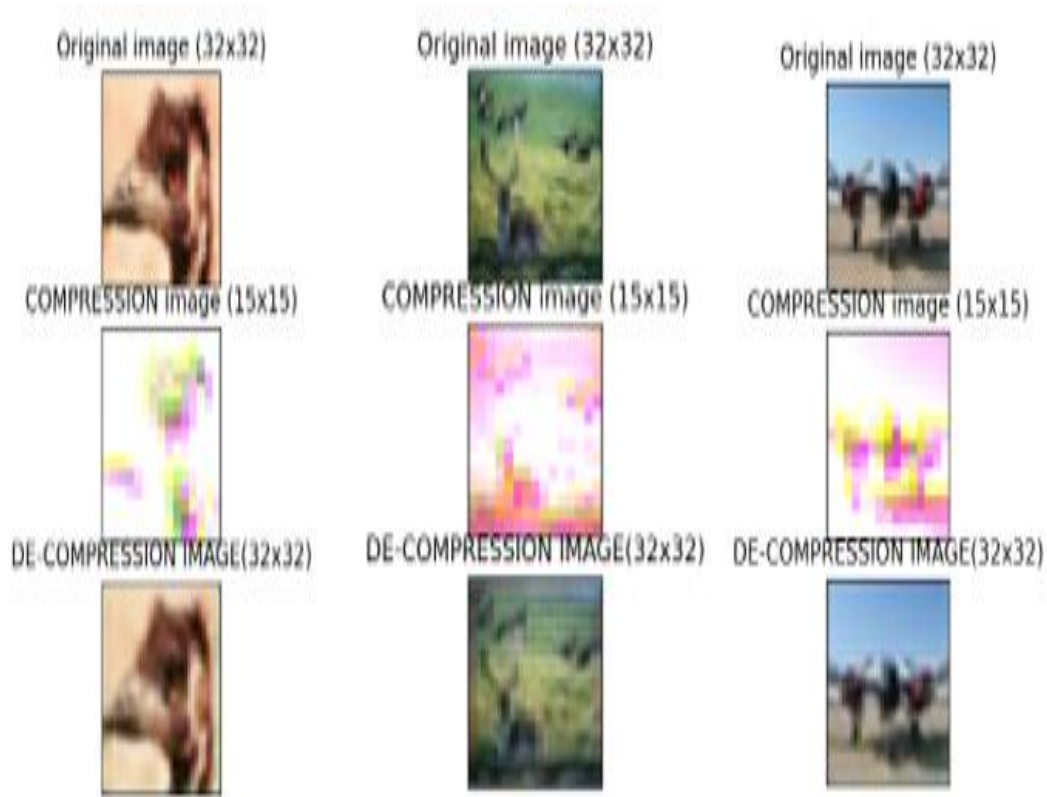
Fig 9. Representing the Reconstruction of Images for CIFAR10 with compression Image with 15x15 with 12.5kb in BMP
